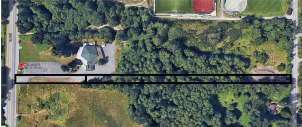
Figure 5: Catchment Areas used for Sizing the Storm Sewer
