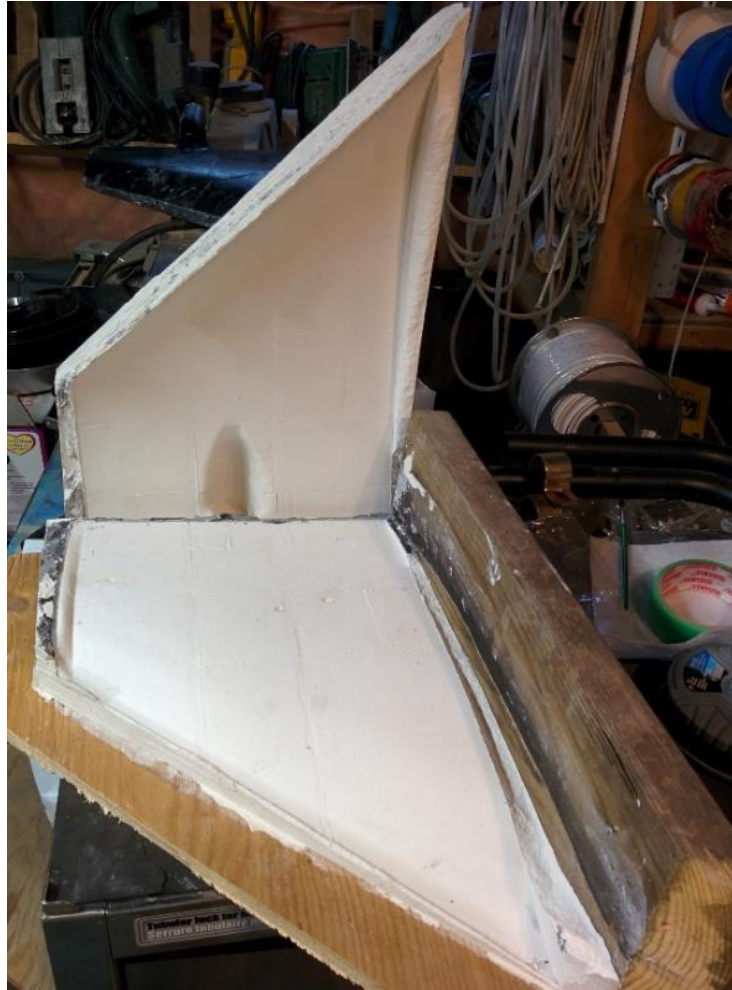
Figure 37: Plaster-mold for Composite Layup
