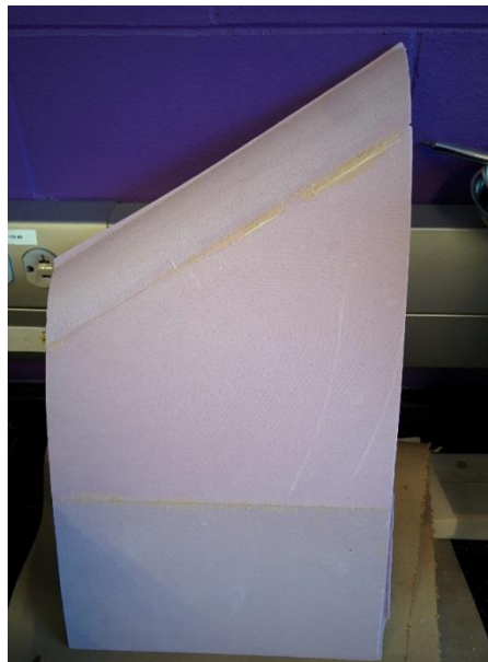
Figure 42: Assembled Foam Mold Sections
