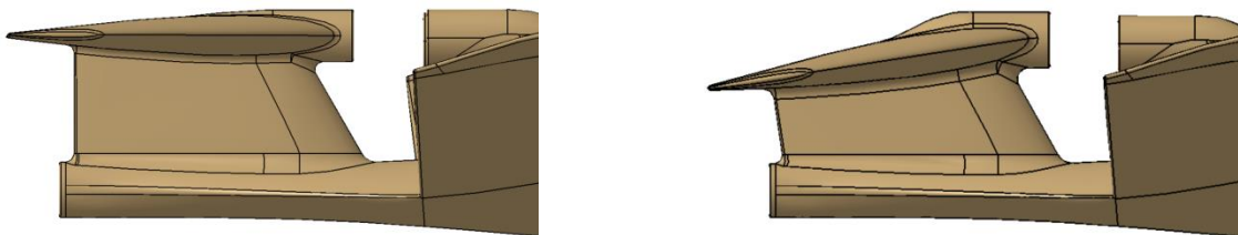
Figure 6: Summary of Old (left) and New (right) Tail Designs
