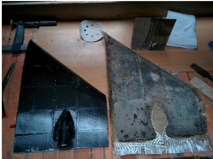
Figure 38: 3D Printed Master (left) and Fiberglass Composite (right)
